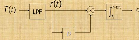
Fig. 2. Receiver for TR-UWB. Note that D(Delay element) can be replaced with a mixer to form FSR.
