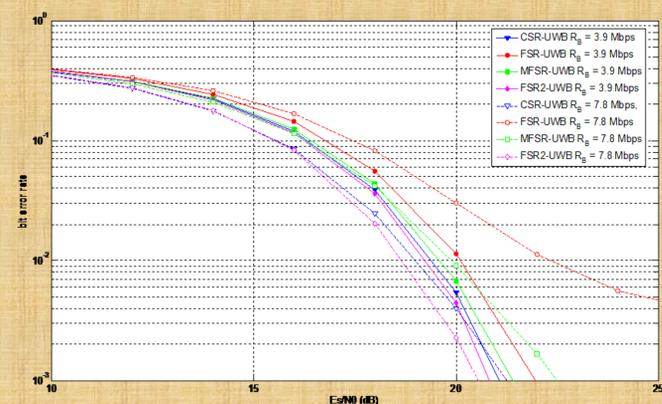
Fig. 5. Performance of various binary schemes on the IEEE 802.5.14a indoor NLOS model (CM4) with a fixed frame time of  $T_f = 16$  ns,  $N_f = 8$  (dashed curves) and  $N_f = 16$  (solid curves) correspond to  $R_b = 7.8$  Mbps and 3.9 Mbps, respectively.
