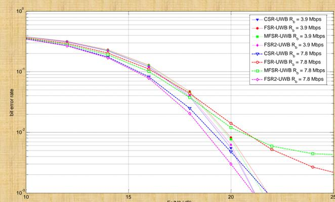
Fig. 4. Performance of various binary schemes on the IEEE 802.5.14a indoor LOS model (CM3) with a fixed frame time of  $T_f = 16$  ns,  $N_f = 8$  (dashed curves) and  $N_f = 16$  (solid curves) which correspond to  $R_b = 7.8$  Mbps and 3.9 Mbps, respectively.
