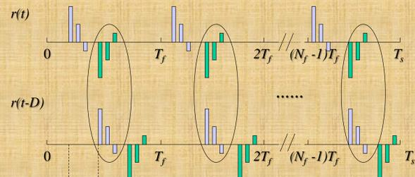
Fig. 1. An example of TR-UWB receiving data bit = -1
