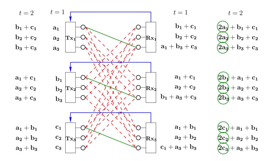
Sum of two-(or more)-codewords should be a codeword. Nested Lattice Codes for interference alignment. Decoding of lattice codeword(s) → cancel off to decode signal.
