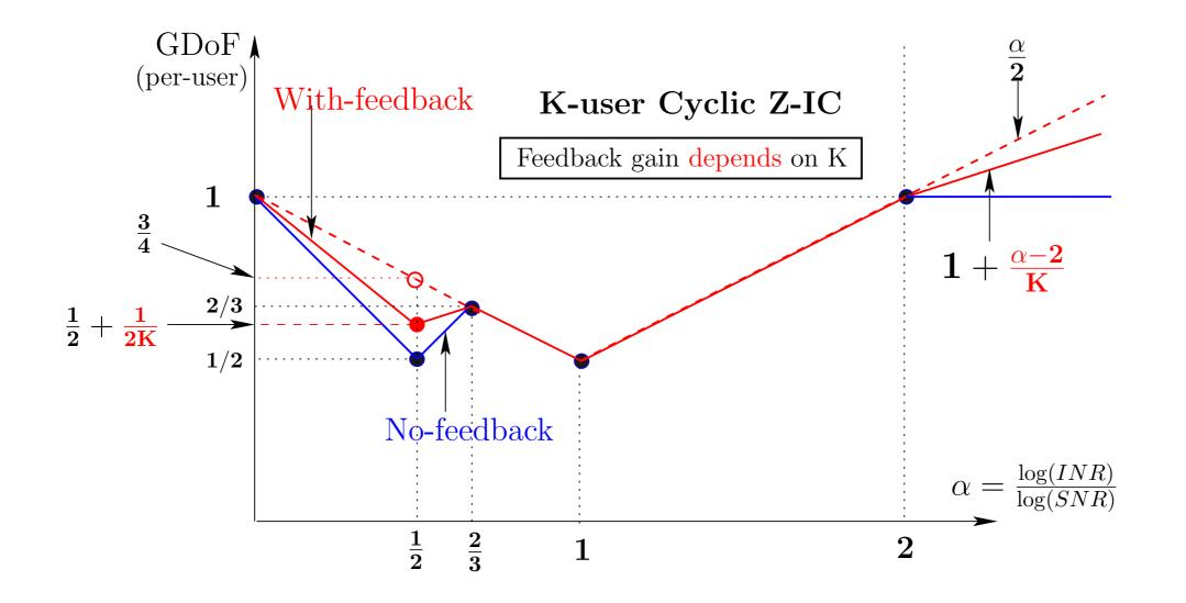
Per-user feedback gain depends on K. As K increases, V-curve → W-Curve
