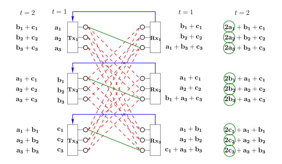
Transmitters decode net-interference viafFeedback Interference at t=2 should be the same as the clean signal at t=1.
