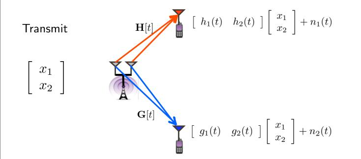
If, in addition to channel state, transmitter also has outputs ... does DoF increase?
